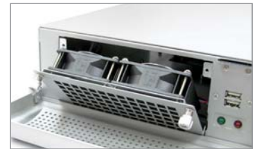
Front Replaceable Air Filters/Fans
