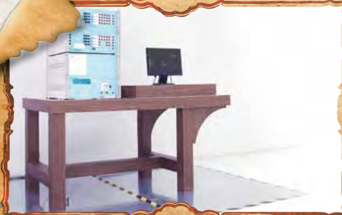
In-house Surge/Dips LAB compliance with IEC 61000-4-5/61000-4-11
