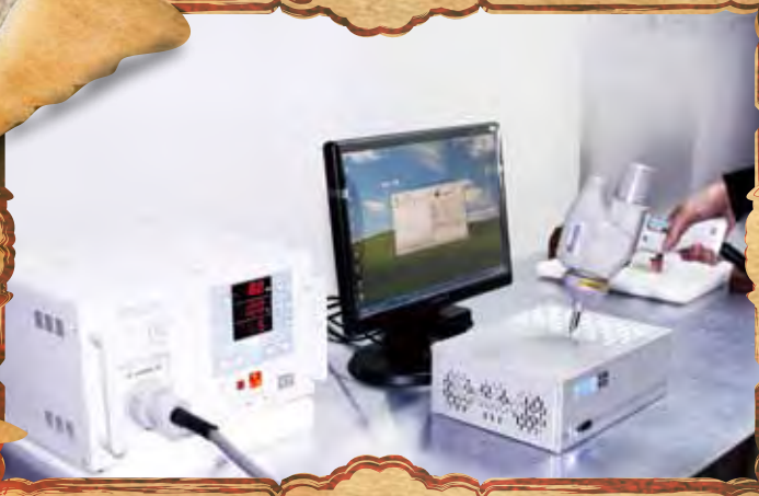
In-house ESD LAB compliance with IEC 61000-4-2
