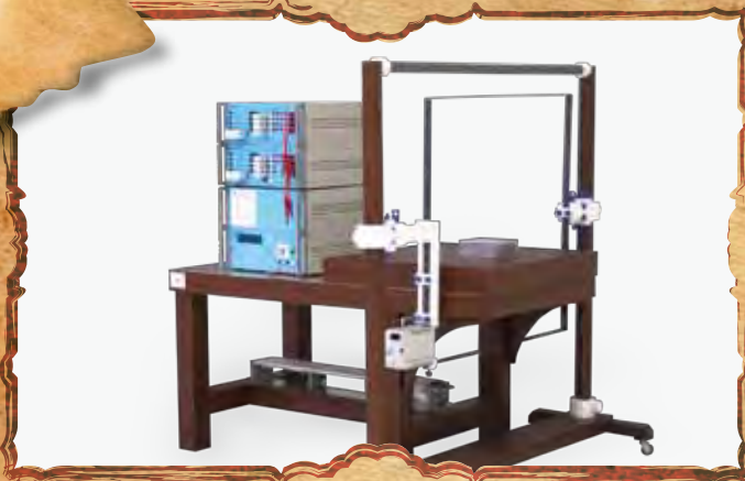
In-house Magnetic Lab compliance with IEC61000-4-8/61000-4-9
