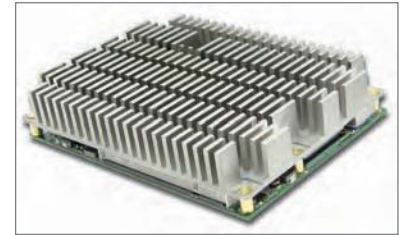
Passive Heat Sink
