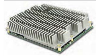
Passive Heat Sink
