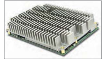
Passive Heat Sink
