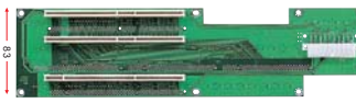
PBP-06V564 Vertical 6-slot (2xPCI-X, 3xPCI) 64-bit PICMG 1.2 Backplane - Fit for 2U chassis - ATX power connector support
