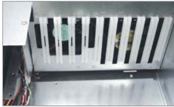
One 12cm and one 8cm Cooling Fans Better ventilation to provide the system with higher reliability
